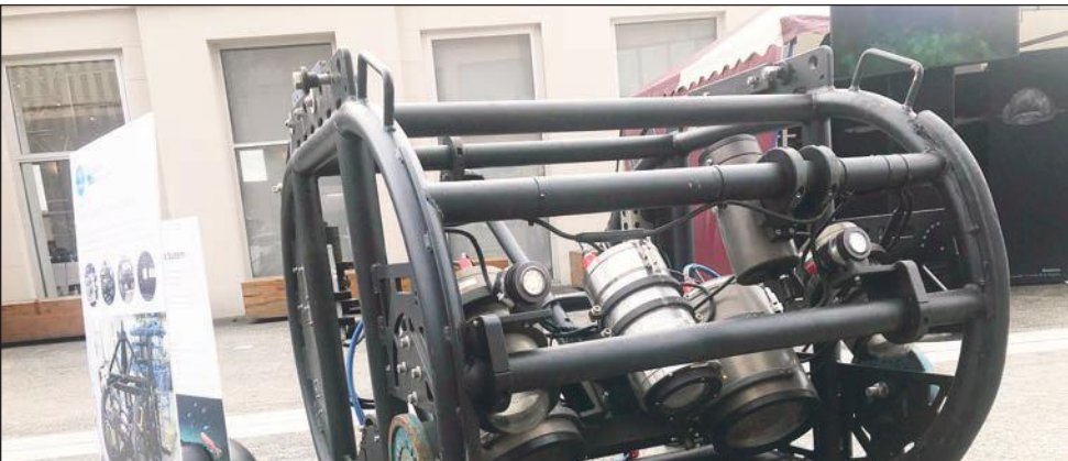
A deep towed camera system used by the CSIRO marine team to capture images and video of features on the ocean floor in depths up to 6000 metres.
