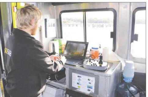
The remotely operated underwater vehicles are piloted by land-based operators who utilise cameras to identify breakages in the nets and conduct repairs. es
